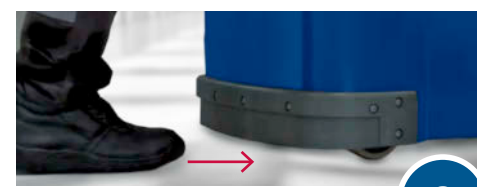
2 Vehicle equipped with foot protection switch. After collision and stop, the vehicle reverses.
