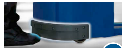
1 Vehicle equipped with foot protection switch. Collision with foot detected. Vehicle stops.
